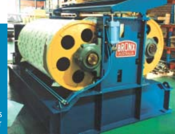
A typical 2 roll bridle - two of these are used on each of the motoring and regenerating bridles.
