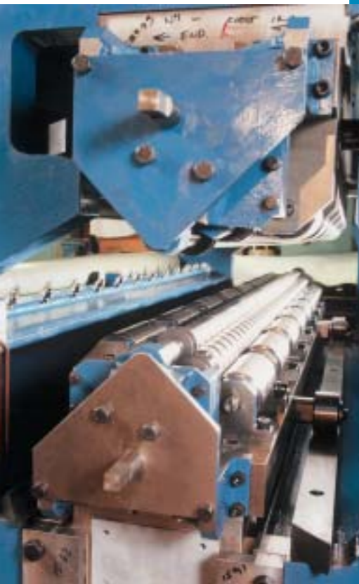
A 6 high cassette used for levelling superior surface quality material.
