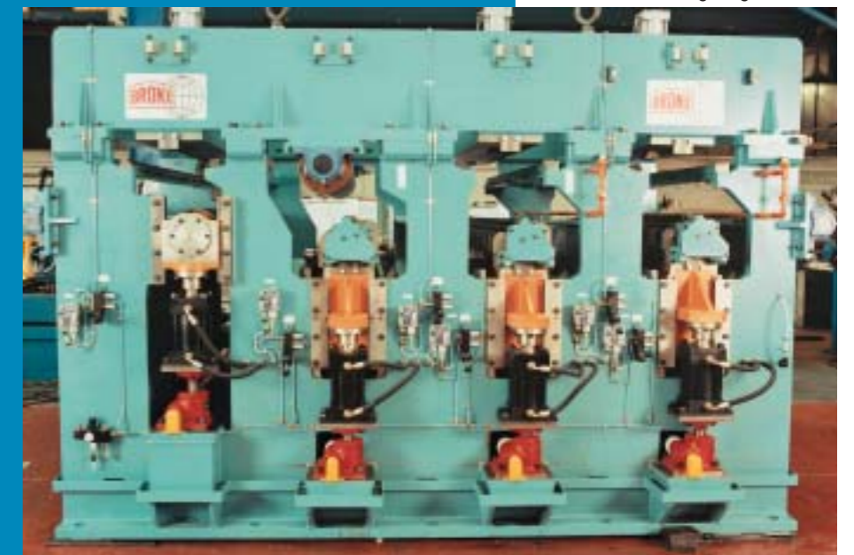
A leveller with two levelling and two de-curving stages.
