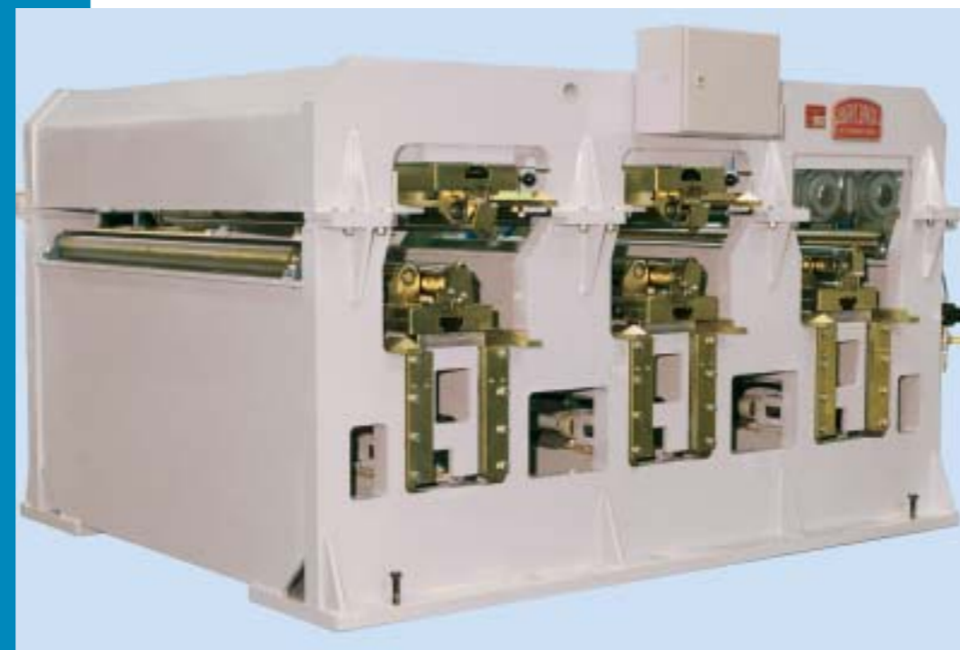
A leveller with two levelling and one de-curving stage.
