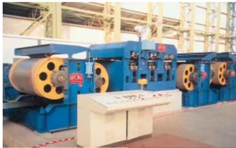
Tension leveller installed in a continuous galvanizing line.
