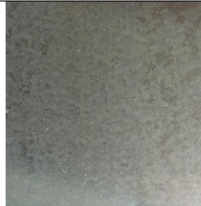
Figure 2. Galfan has a smooth reflective surface with faint hexagonal boundaries.
